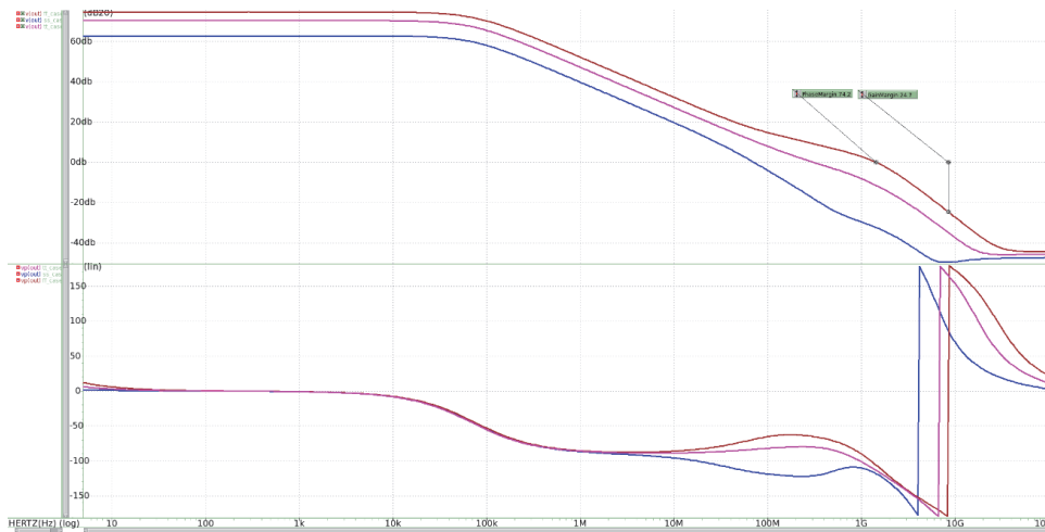
Fig. 3. The AC characteristic of the designed folded-cascode op-amp
