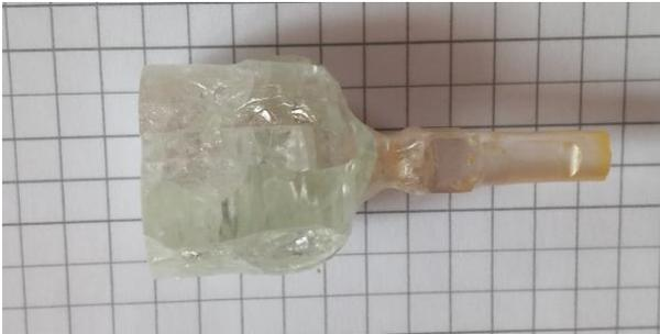
**Fig. 2.**  $\text{LiNb}_{0.88}\text{Ta}_{0.12}\text{O}_3$  crystal grown by conventional Czochralski method.
