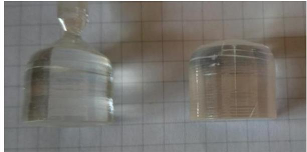
**Fig. 3.**  $\text{LiNb}_{0.88}\text{Ta}_{0.12}\text{O}_3$  crystal grown by Czochralski method with a very low pulling rate.
