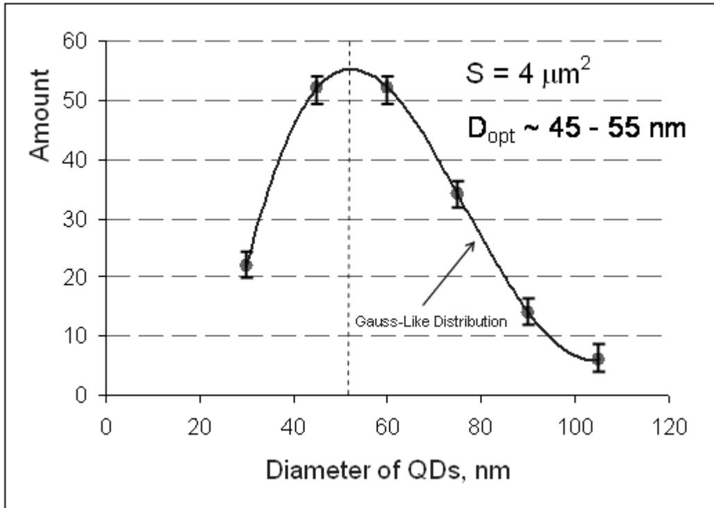
**Fig. 2.** Dependence of the InAsSbP QDs amount versus their average diameter.
