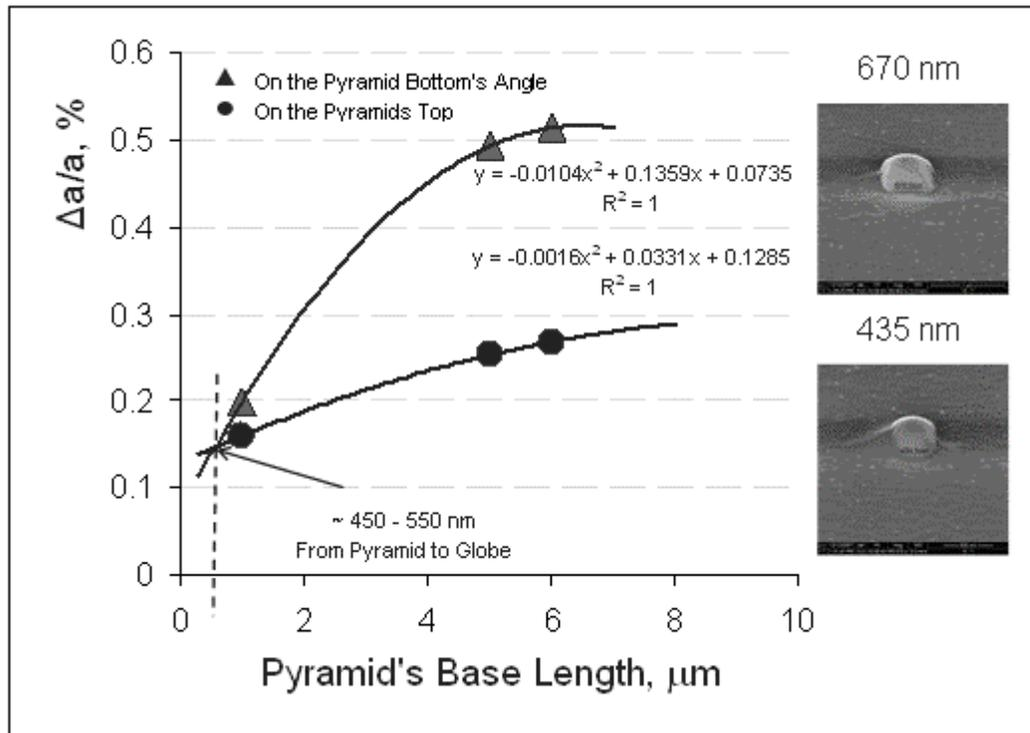
**Fig. 4.** Dependence of lattice mismatch ratio on the bottom and top of InAsSbP-based strain induced pyramids versus to their base length.
