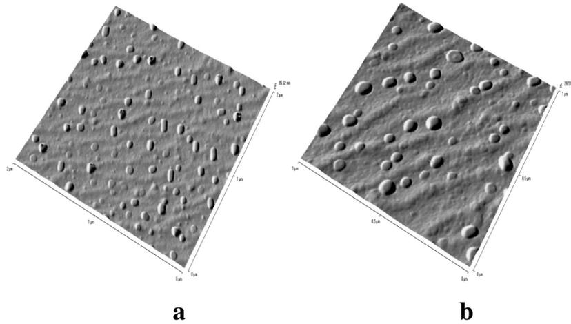
**Fig. 1.** The oblique view of AFM images of InAsSbP QDs grown by liquid phase epitaxy on InAs (100) substrate, a –  $S=2 \times 2 \mu\text{m}^2$ , b –  $S=1 \times 1 \mu\text{m}^2$ .
