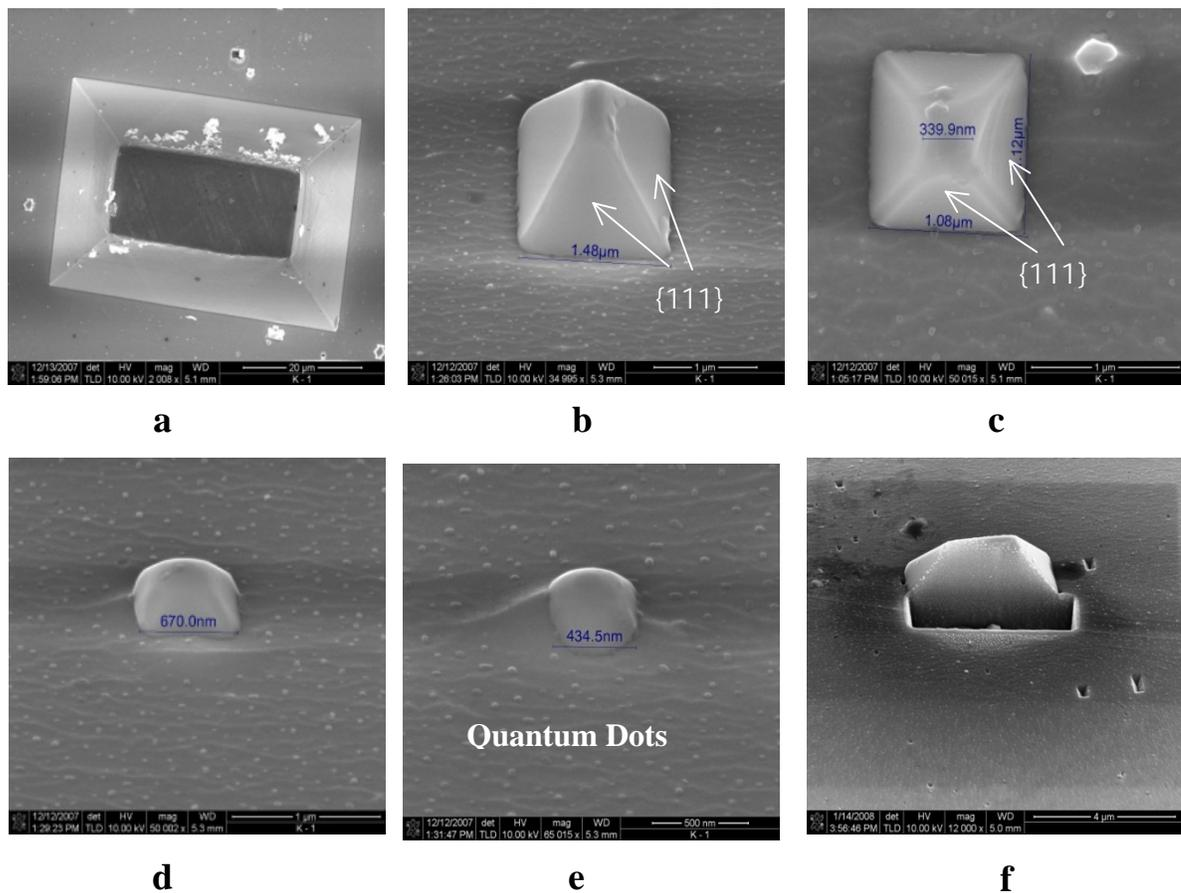
**Fig. 3.** The self-assembled InAsSbP-based strain-induced islands grown by liquid phase epitaxy on InAs substrate and their evolution from the pyramid to globe – a, b, c, d, e; f – pyramid cut by Focused Ion Beam.
