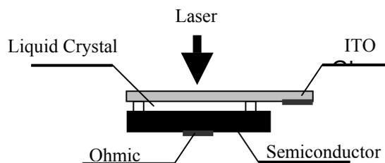
Fig. 1. Design of liquid crystal semiconductor cell.
