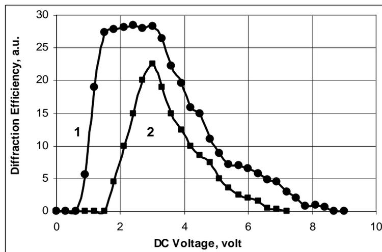
Fig. 5. Diffraction efficiency vs. dc voltage for the sample with the silicon substrate (1) and with two ITO-coated glass substrates (2).
