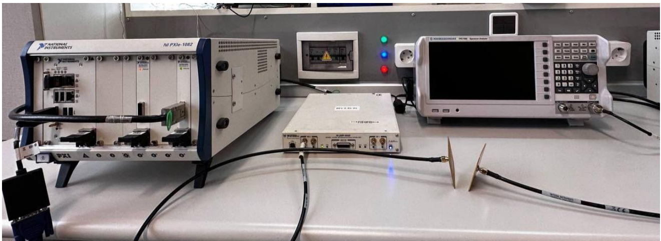
Fig. 1. Laboratory measurement configuration for DSB-SC signal transmission and spectral analysis, including the PXIe-1082 control chassis, USRP-2954 SDR transmitter, TX antenna, and Rohde & Schwarz spectrum analyzer.
