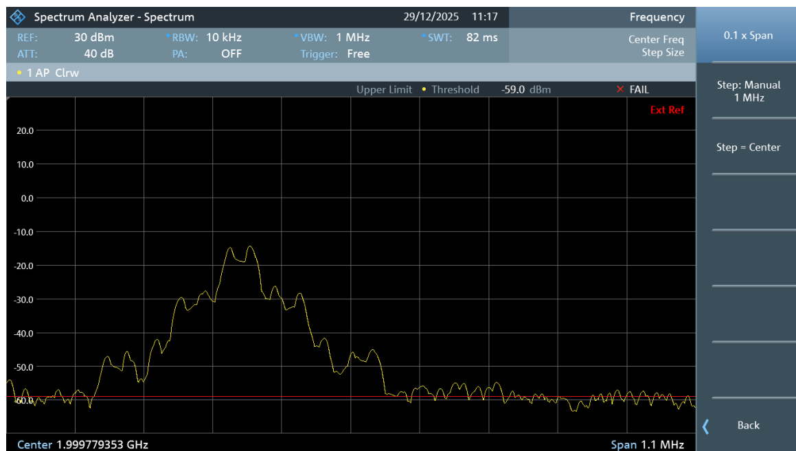
Fig. 2. Measured RF spectrum of the transmitted SC-DSB signal centered at approximately 2 GHz (RBW = 10 kHz, VBW = 1 MHz, span = 1.1 MHz).
