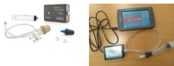
Picture. Equipments for determining root pressure using the LabQuest 2 device.
