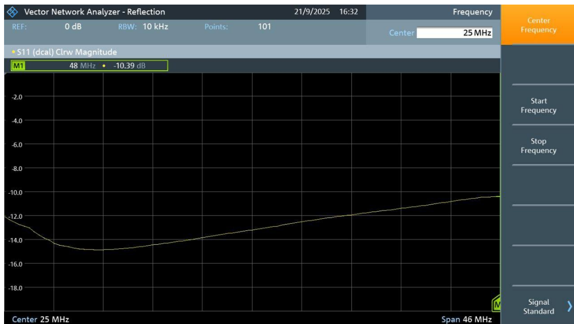
Fig. 2. Standing wave ratio (SWR) / reflection coefficient (S11) measurement of the applicator antenna.
