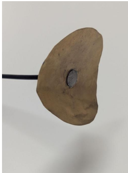
Fig. 1. Applicator antenna used for registering brain-origin RF signals. The sensor consists of a metallic electrode connected via coaxial cable, a dielectric layer for safe contact, and a protective shielding electrode to minimize external interference.
