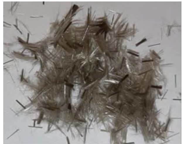
Fig. 1. Dispersed basalt fibers for cement mortar reinforcement
