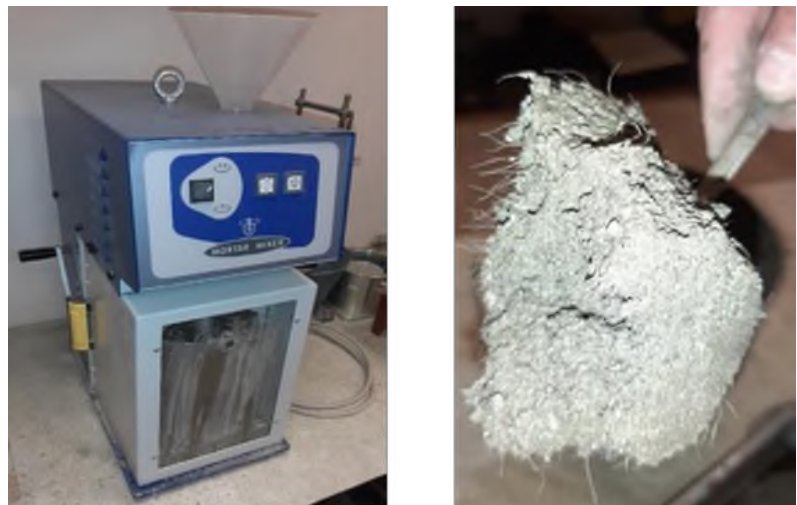
Fig. 2. Electric mixer (a) for mortar and the resulting fiber mixture (b)
