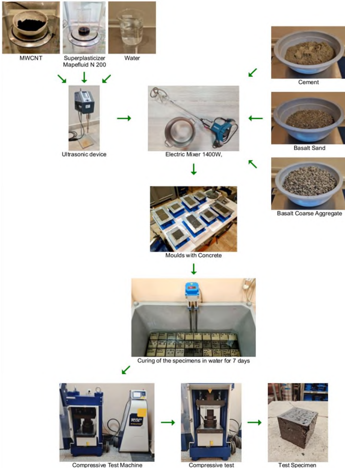
Fig. 2. Sample preparation steps, curing and testing processes
