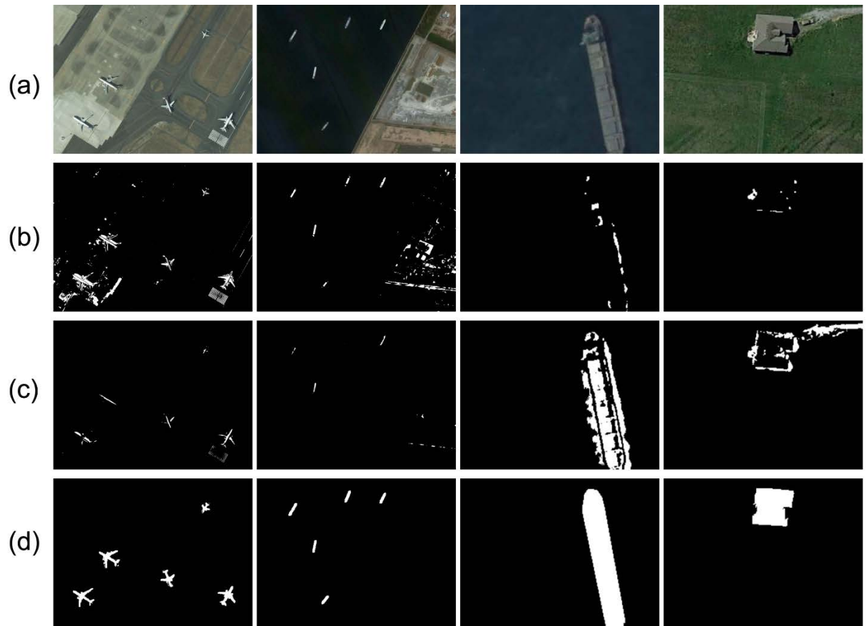
Fig. 4. Spectral residual saliency (SRS) detection: (a) input image, (b) output of SRS w/o enhancement, (c) output of SRS after enhancement, (d) ground-truth mask.
