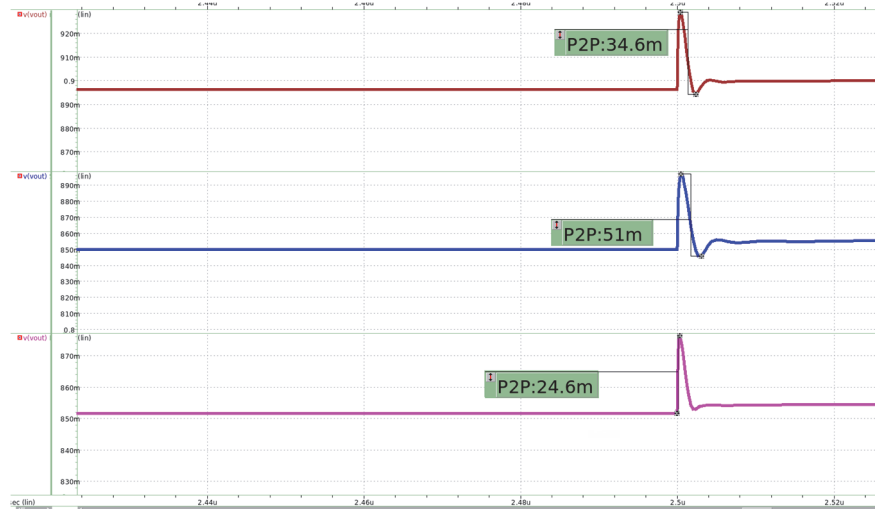
Fig.12. Voltage regulator output voltage with proposed architecture
