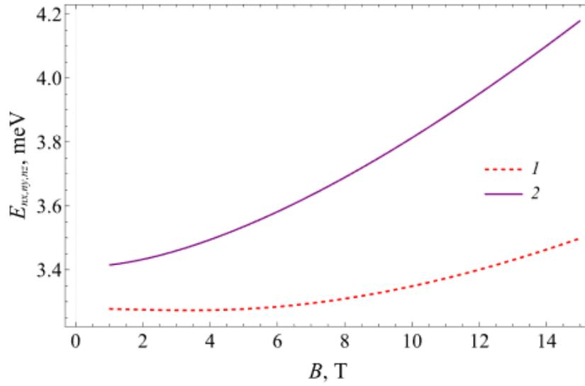
**Fig. 3.** The system's energy  $E_{n_x, n_y, n_z}$  dependence on the magnetic field  $B$ , for the fixed values of geometrical parameters  $a = 5a_B, b = 7a_B$  and  $c = a_B$ . The energy levels considered are:  $\{n_x, n_y, n_z\} = \{1, 2, 1\}$  (curve 1),  $\{n_x, n_y, n_z\} = \{2, 1, 1\}$  (curve 2).
