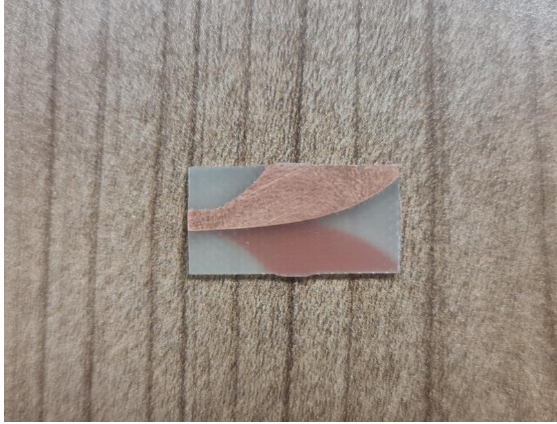
Fig. 2. Fabricated antipodal Vivaldi antenna without source connector.
