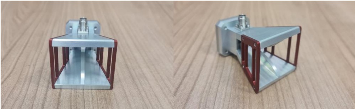
Fig. 4. Double-ridged horn antenna for PNFR system validation.
