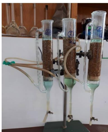
Fig.4. Biolaching of oxidized ore by “Kashen” consortia: 1 - control without bacteria, 2, 3-uninoculated by “Kashen” consortium (PD- 150: 120, pH 1.3, at room temperature)
