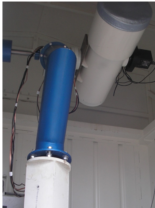
Figure 5. 250 mm aperture telescope mounted in the container-dome.
