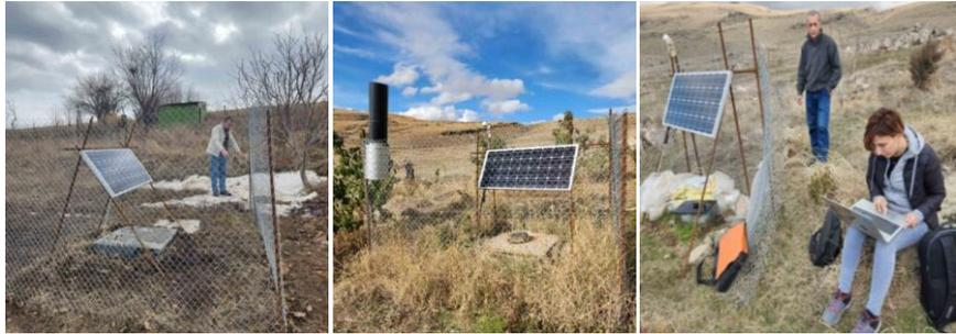
**Fig.2.** The installation and service of three temporary seismic stations.
