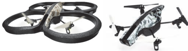
Fig. 4. AR.Drone 2.0 with Indoor and OUT hulls
