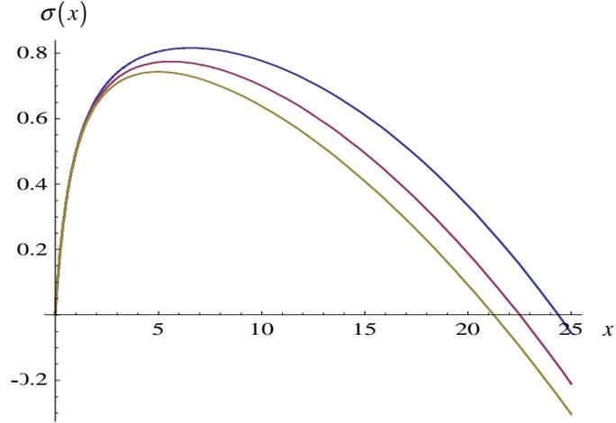
Fig 2. The stress states for three different space elevator tubes.
