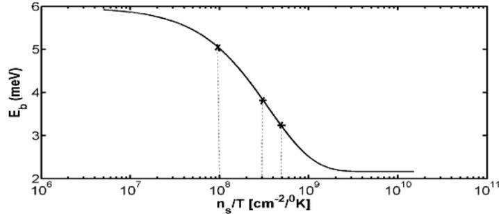
**Fig. 1.** The binding energy of the screened exciton  $E_b$  as the function of density / temperature ratio parameter  $n_s/T$  in the cases of QW width  $d=10\text{nm}$  ( $10^6 \div 10^8 \text{ cm}^{-2}/^\circ\text{K}$ ),  $d=5\text{nm}$  ( $10^6 \div 2 \cdot 10^8 \text{ cm}^{-2}/^\circ\text{K}$ ),  $d=3\text{nm}$  ( $10^6 \div 4 \cdot 10^8 \text{ cm}^{-2}/^\circ\text{K}$ ) and  $d=1.5\text{nm}$  ( $10^6 \div 10^{12} \text{ cm}^{-2}/^\circ\text{K}$ ).
