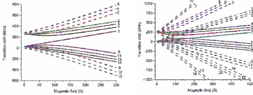
Fig. 2. Magnetic field dependence of the energy shifts of the <sup>41</sup>K isotope D<sub>1</sub> (left) and D<sub>2</sub> (right) lines. The solid lines describe the transitions which exist in HPB regime, while dashed lines describe transitions whose probabilities tend to zero in HPB regime. The zeros are  $F=2, m_F=-1$  to  $F'=1, m_F=-1$ .
