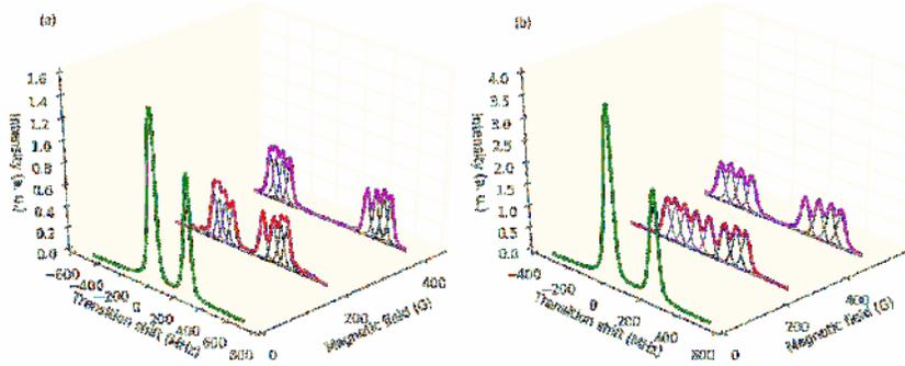
Fig. 4. Spectra of  $^{41}\text{K}$  (a)  $D_1$  line; (b)  $D_2$  line for  $B = 0\text{G}$ ,  $B = 200\text{G}$  and  $B = 400\text{G}$  magnetic fields. The zeros are  $F=2, m_F=-1$  to  $F^I=1, m_F=-1$ .
