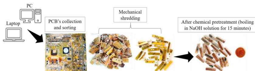
Fig. 1. View of shredded PCBs after: dismantling and components removal (a), being cut (b) and chemical pretreatment (c)
