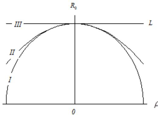
**Fig. 3.** Equiphase curves of a spherical wave (I) on the plane  $R_0, \rho$ , Fresnel (II) and Fraunhofer (III) approximations, respectively.
