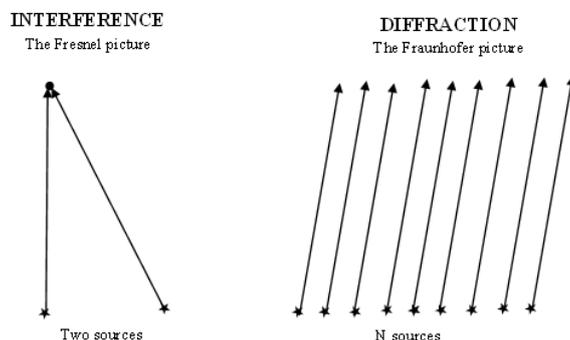
**Fig. 1.** Interference of waves from two sources (near observation region) and diffraction of waves from  $N$  sources (far observation region).
