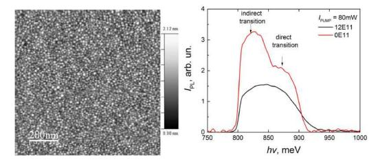
Figure 1. AFM image of Ge/Si QDs (on the left). PL spectra for different impurity concentration (on the right).
