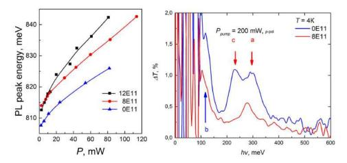
Figure 2. Dependence of the PL peak on the pump power (on the left). Photoinduced absorption spectra at the same pumping and different impurity concentration (on the right).
