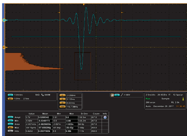
Fig. 4: Scope Charge measurement Q =33 pC FC out.
