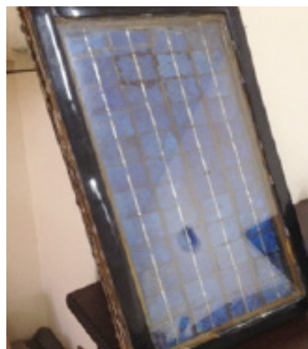
Figure 3. Desalination device with integrated PV panel.
