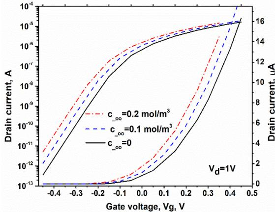
Fig. 3. The drain current versus gate voltage at different species concentration.
