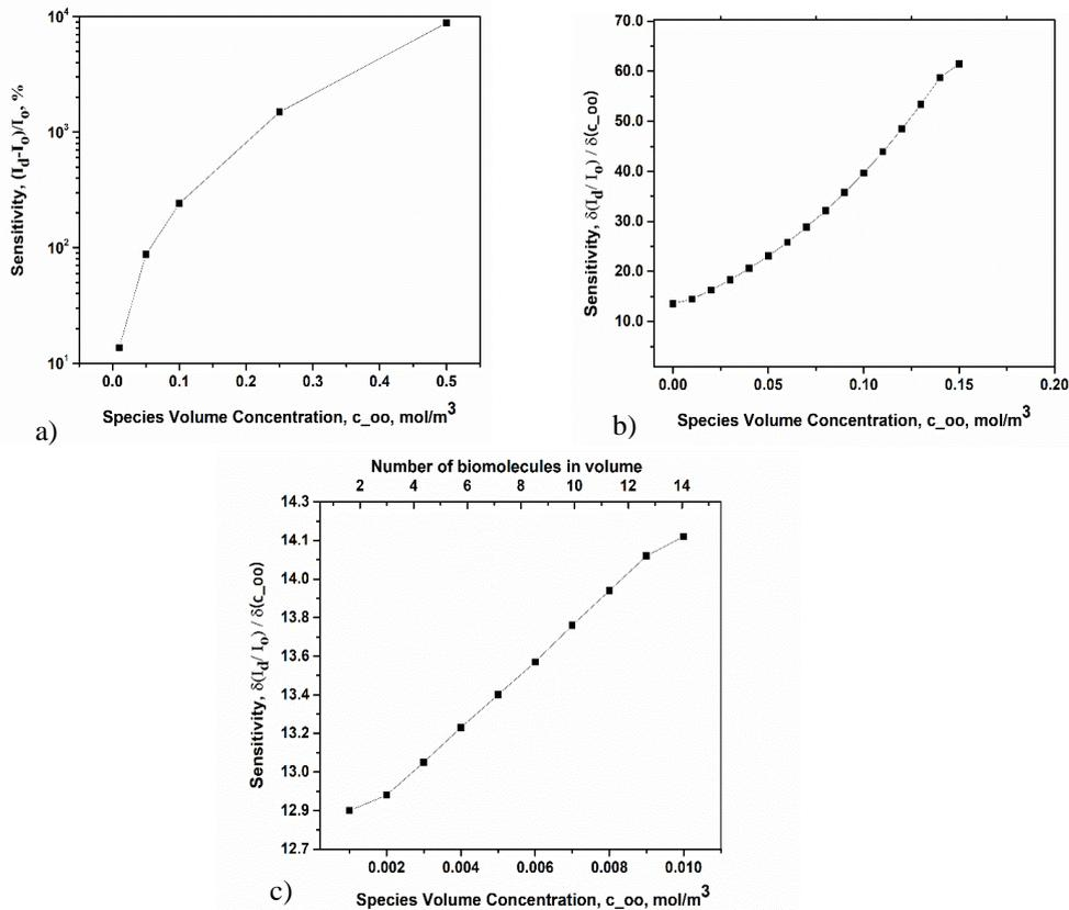
Fig. 5. The NW sensor sensitivity versus species volume concentration.
