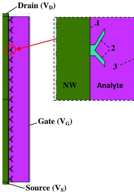
Fig. 1. The cross section of modeled structure.
