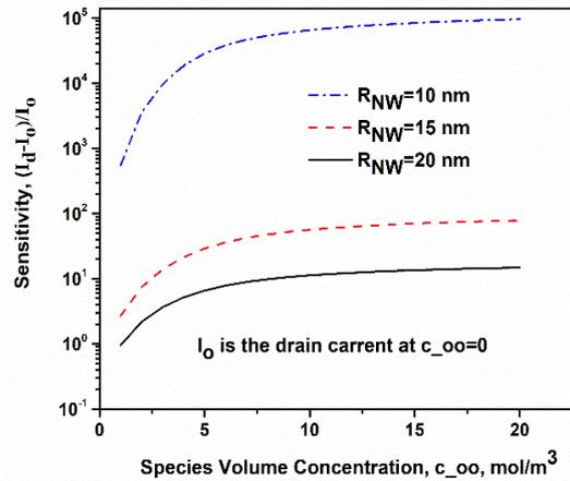
Fig. 4. The NW sensor sensitivity versus species volume concentration at different NW radii.
