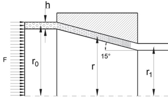
Fig. 1. The scheme of thin-walled pipe extrusion
