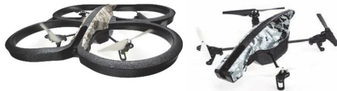
Fig. 4. AR.Drone 2.0 with Indoor and OUT hulls
