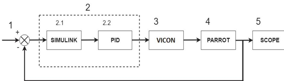
Fig. 5. Block diagram of the Parrot control system
