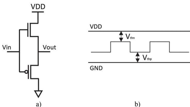
Fig. 6. a- Process-relative signal generator, b- Process detection
