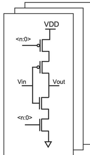
*Fig. 7. The VCO cell of the purposed system*
