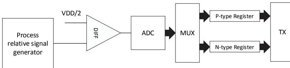
Fig. 3. The structure of the process compensation method
