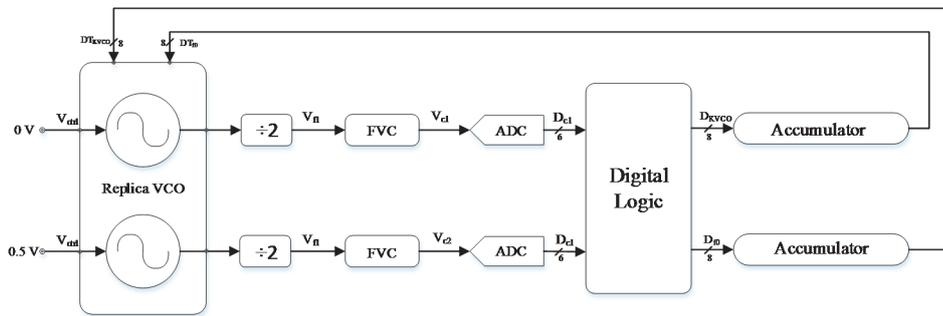
Fig. 2. The block diagram of the calibration system
