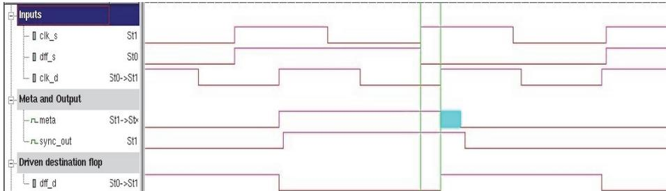
Fig. 3. The synchronizer cell model simulation waves 1
