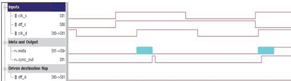
Fig. 4. The synchronizer cell model simulation waves 2
