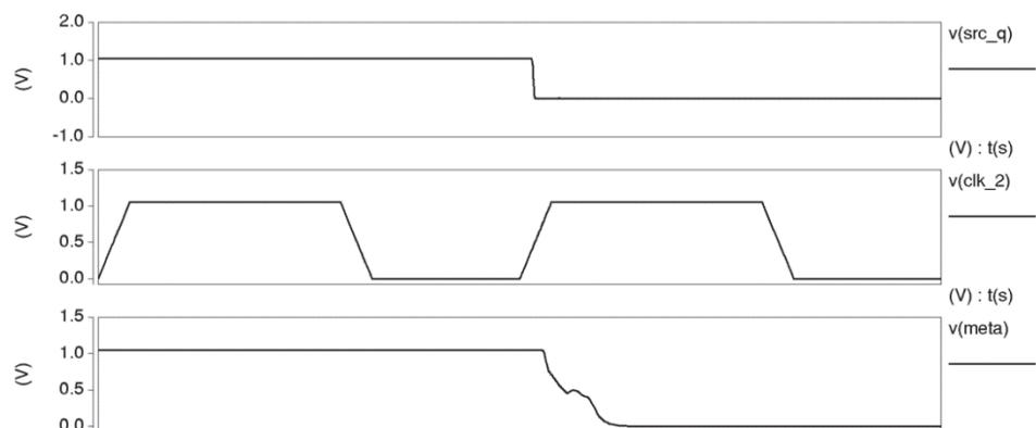
Fig. 1. A metastability simulation example
