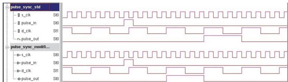
Fig. 6. Comparison of a standard pulse synchronizer
