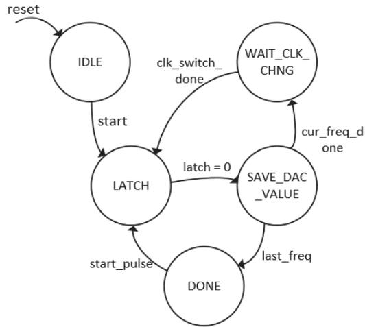
Fig. 3. FSM of the digital calibration logic
