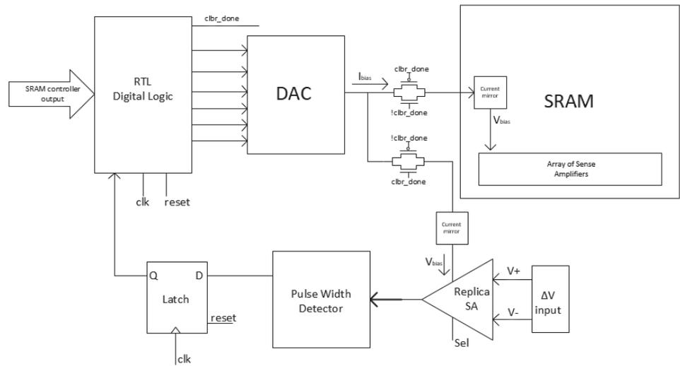
Fig. 2. The block diagram of SCU for SRAM
