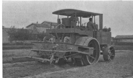
The Nubari Plowing Machine. Source: "An Egyptian Steam Cultivator," Scientific American , February 13, 1909
