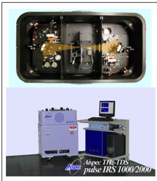
Fig.2 Photographic view of the air evacuated bench unit (upper) of the newly developed versatile THz-TDS instrument. Aispec model: pulse IRS 2000/2000 (lower).
