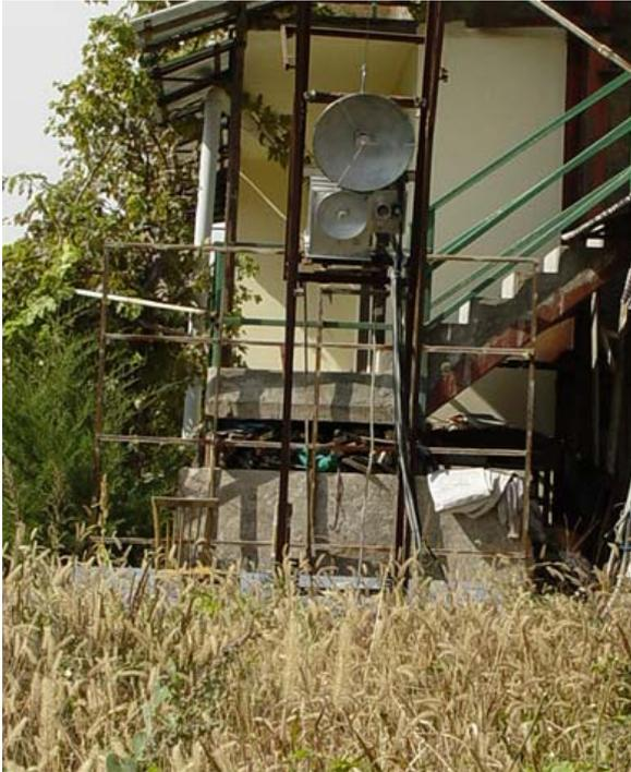
Fig. 3 The CSRS at 5.6GHz, 15GHz and 37 GHz set on the mobile buggy at the bottom of the platform
