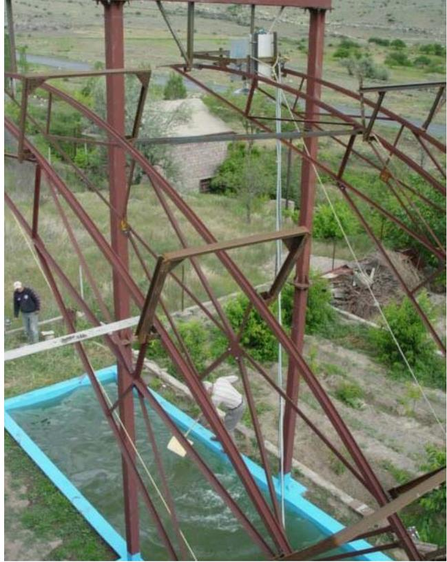
Fig.2 ArtAr-5.6, ArtAr-15 and ArtAr-37 CSRS set on the mobile buggy at the top of the measuring platform
