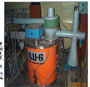
The main component of the RF system is the microwave source. There is a variety of microwave tubes for generating and amplifying microwave signals. The two most common used in linacs are magnetrons and klystrons. Rf linear electron accelerator contain some part such as: electron gun, rf system, acceleration tube, vacuum system, cooling system, magnet system , beam line contain scanning magnet and horn .figure 3 show the one kind of rf industrial linac [3,4,6-8].
