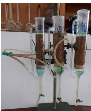
**Fig.4.** Bioleaching of oxidized ore by “Kashen” consortia: 1- control without bacteria, 2, 3-uninoculated by “Kashen” consortium (PD- 150: 120, pH 1.3, at room temperature)
