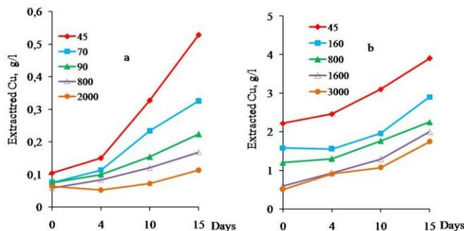
**Fig.1.** Effect of particle size on bioleaching of copper by “Kashen” consortium from sulfide (a) and oxidized (b) ores of Kajaran deposit (PD – 20%, pH –1.8; t – 35<sup>0</sup>C, 180 rpm)
