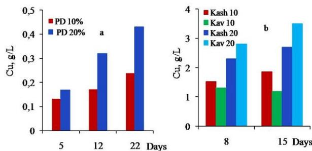
**Fig.2.** Recovery of copper from sulfide ore by “Kashen” consortium (a) and oxide ore by “Kashen” and “Kavart” consortia at pulp density of 10 (Kash 10, Kav 10) (b) and 20 % (Kash 20, Kav 20) (b) (PS – 63  $\mu\text{m}$ , t – 30  $^{\circ}\text{C}$ , 160 rpm)
