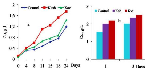
**Fig.3.** Biorecovery of copper from sulfide (a) and oxidized (b) ore samples by adapted consortia “Kashen” and “Kavart” (PD-20 %,  $t$  - 30 °C, 160 rpm)
