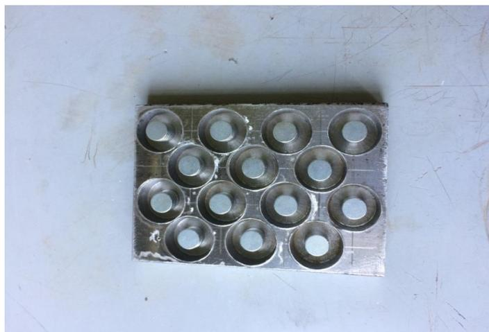
**Fig. 9.** Block of round minimagnetrons
