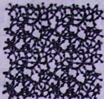
FIG 1. The structure of amorphous silicon dioxide ( \alpha - \text{SiO}_2 ) is described by 3D random network with covalent bonds.
