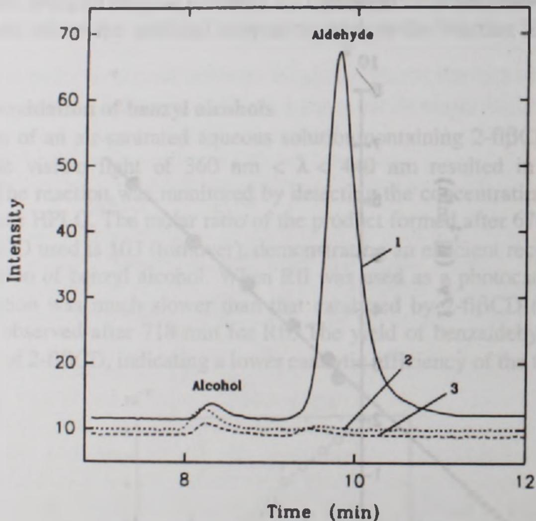
**Figure 5.** HPLC Chromatograms for Analysis of the Reaction Mixture in the Oxidation of p-t-Butylbenzyl Alcohol by Flavins. 1. catalyzed by 2-fl $\beta$ CD for 53 min. 2. catalyzed by Rfl for 51 min; 3. catalyzed by Dmfl for 76 min.
