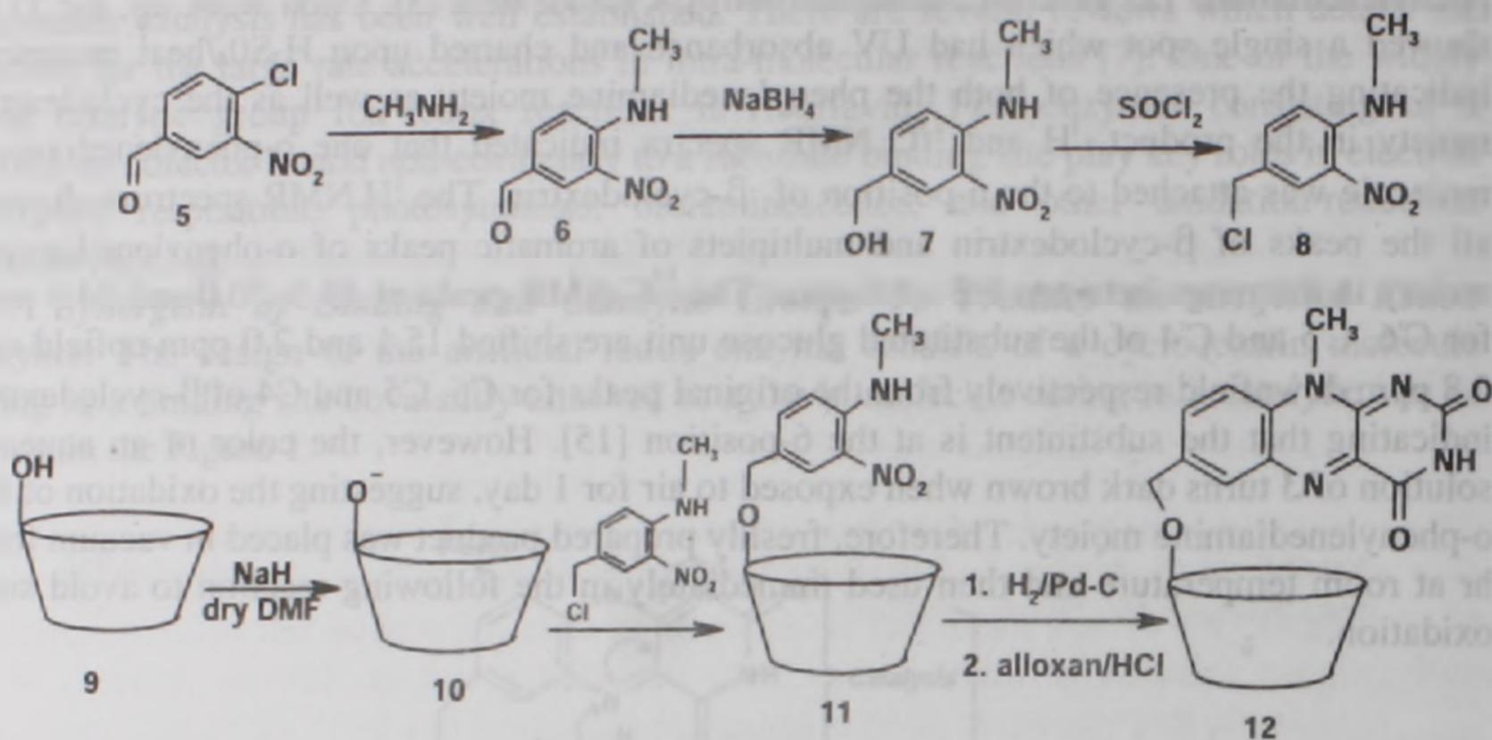
Scheme 2. Attachment of flavin to the secondary side of cyclodextrins.
