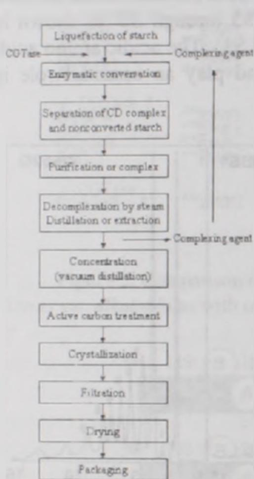
Figure 6. Solvent process for production of cyclodextrin
