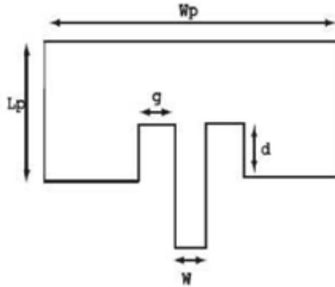
Fig.1 Geometrical view of resonator
