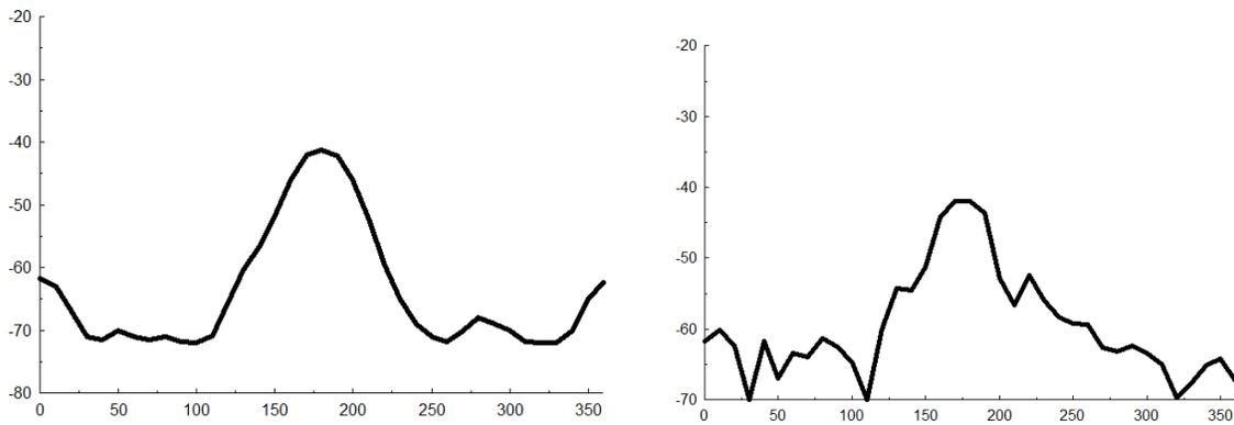
**Fig.6.** The DP of the subarray on the horizontal and vertical planes respectively
