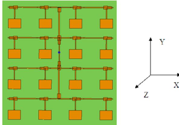
**Fig.3.** General view of subarray in CADFEKO interface
