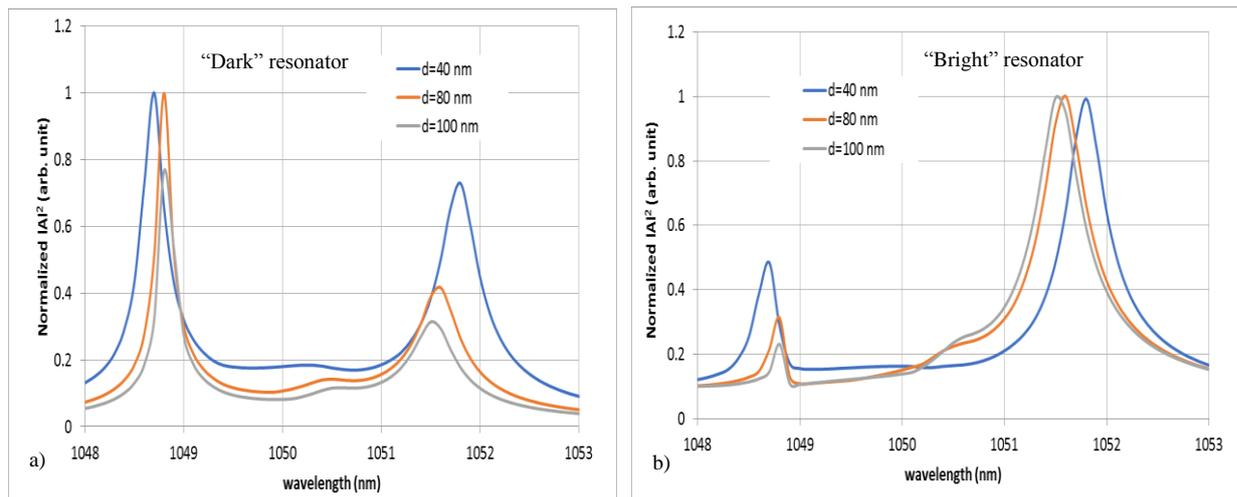
**Fig.3.** Electrical field  $E_z$  component normalized amplitude vs. wavelength a) in “Dark” and b) in “Bright” resonators, for different  $d$  distances between resonators.
