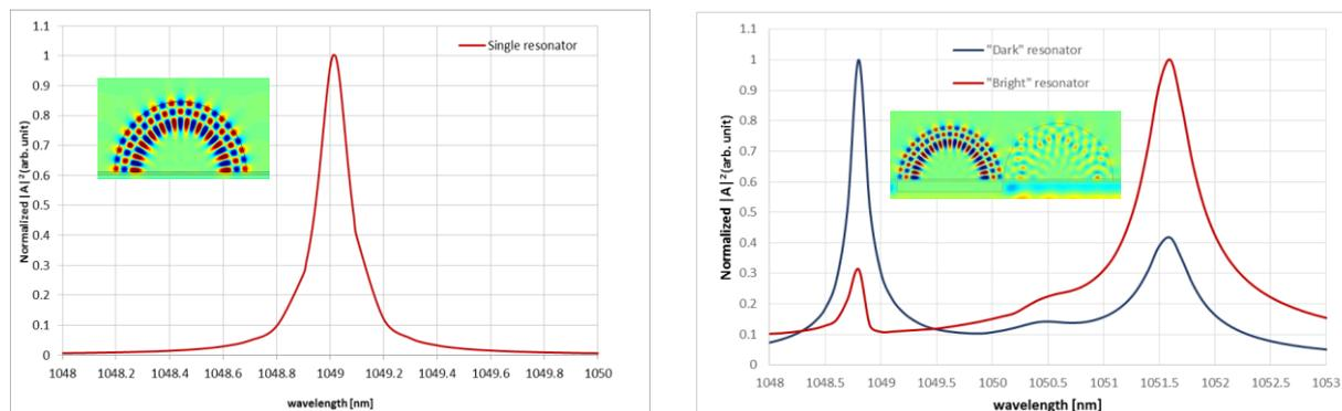
**Fig.2.** Electrical field  $E_z$  component normalized amplitude vs. wavelength for coupled resonators.
