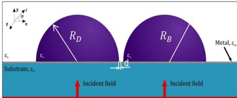
**Fig. 1.** The cross section of the structure of coupled semicylindrical microresonators with different radii.  $\epsilon_d = 2.25$ ,  $\epsilon_e = 1$  are dielectric permittivities of the substrate (SiO2 Silica) and the surrounding medium (Air), respectively. As a metal and semicylinder medium Ag and GaAs ( $\epsilon_s$ ) were used correspondingly.
