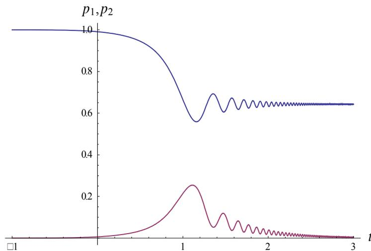
Fig. 2. Occupation probabilities for the ground (upper line) and excited (lower line) states for field parameters  $U_0 = 0.3$  and  $\delta_{0,1} = 1, -5$  ( $\lambda = 0.144$ ).
