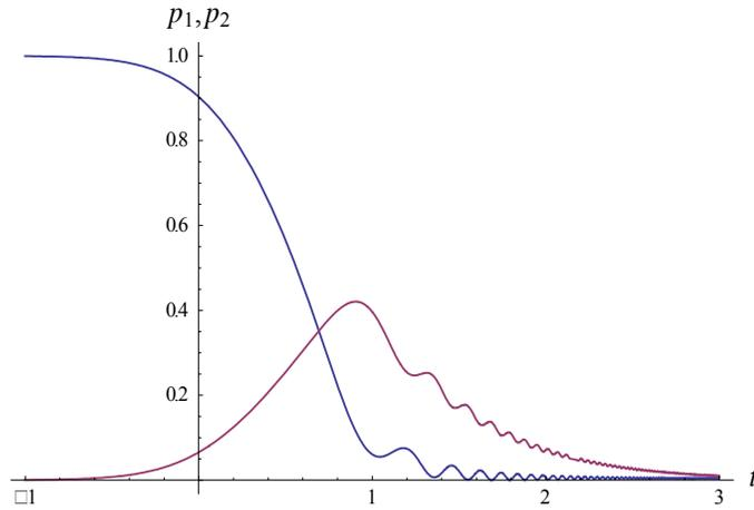
Fig. 3. Occupation probabilities for the ground and excited states (blue and magenta lines, respectively) for field parameters  $U_0 = 1$  and  $\delta_{0,1} = 1, -5$  ( $\lambda = 1.6$ ).
