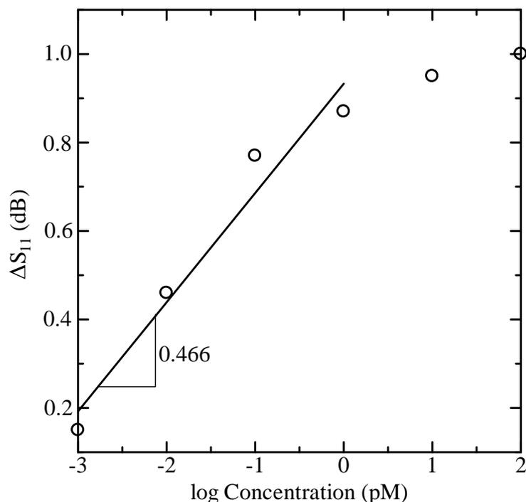
**Fig. 3.** The microwave reflection coefficient change,  $\Delta S_{11}$  as a function of the target concentration of the 10mer oligonucleotide at the resonant frequency.
