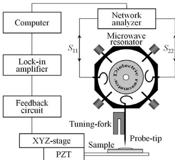
**Fig. 1.** The schematic of NSMM experimental setup.
