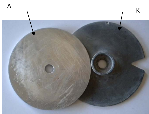
Fig. 1. The external appearance of aluminum electrodes after passing the electric current through the electrolyser, A is the anode, K is the cathode.
