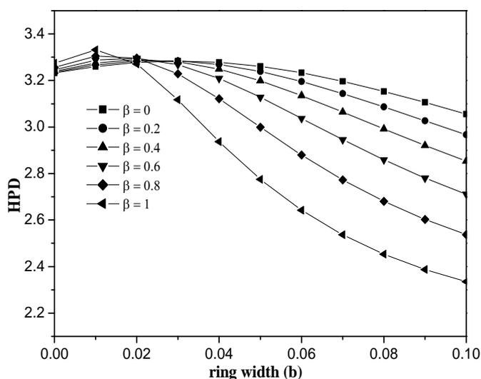
**Fig. 4.** HPD (Half Power Diameter) as function complex pupil filter of ring width ( $b$ ) for different values of  $\beta$ .
