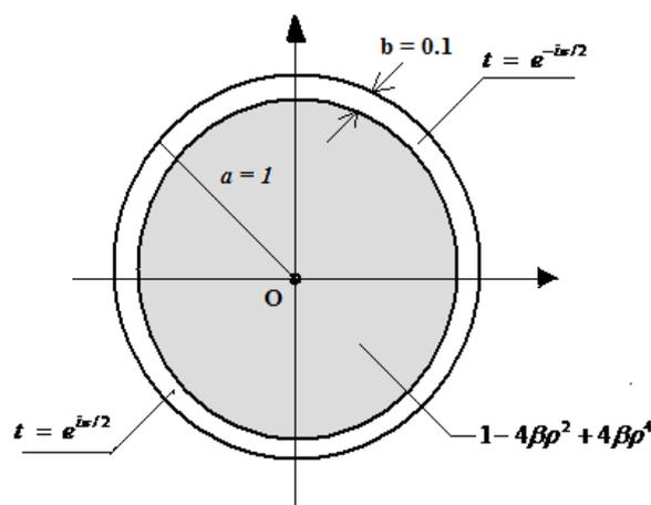
Fig. 1. Structure of three-zone complex pupil filter.
