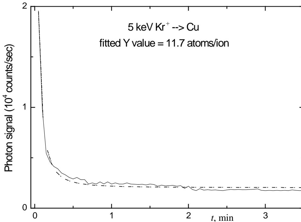
Fig. 2 - Photon yield of the Cu 324.8 nm line versus time of bombardment.
