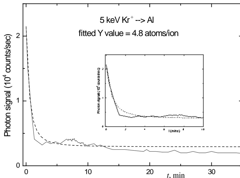
Fig. 1 – Photon yield of the Al 309.3 nm line versus time of bombardment.
