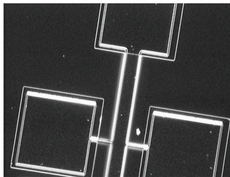
Fig. 1.22. Optical microscope image of p<sup>+</sup>-GaAs/n-GaAs/n<sup>+</sup>-GaAs solar cells monolithically integrated on silicon substrate with high crystallographic index after fabrication of ohmic contacts
