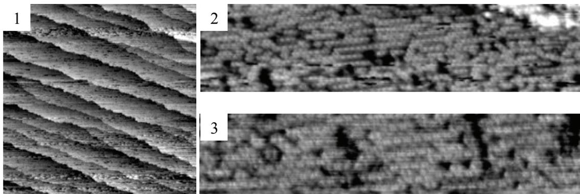
Fig. 1.5. The STM images of Si(113)-3×2 surface with Ge coverage after 2 minutes' deposition at 430°C sample temperature. The scan areas are 500 nm × 500 nm (1), 70 nm × 17 nm (2), 43 nm × 8 nm (3) using sample voltage of -2 V and tunneling current of 0.3 nA.
