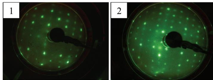
Fig.1.2. The Lof Si(113)-3×2 reconstruction. Electron energies are 40 eV (1), 75 eV (2).
