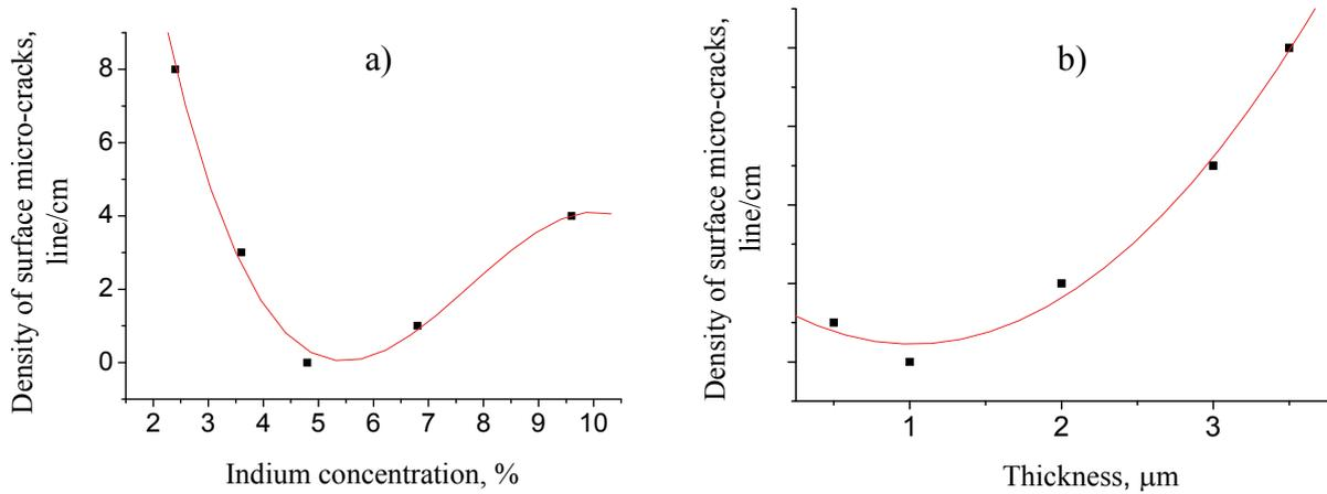
Fig. 1.17. Dependence of the density of surface micro-cracks on indium concentration (a) and thickness (b) of  $\text{In}_x\text{Ga}_{1-x}\text{As}$  buffer layer
