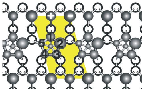
Fig. 1.9.  $2 \times 2$  model of Ge atomic structure on the Si(113) surface
