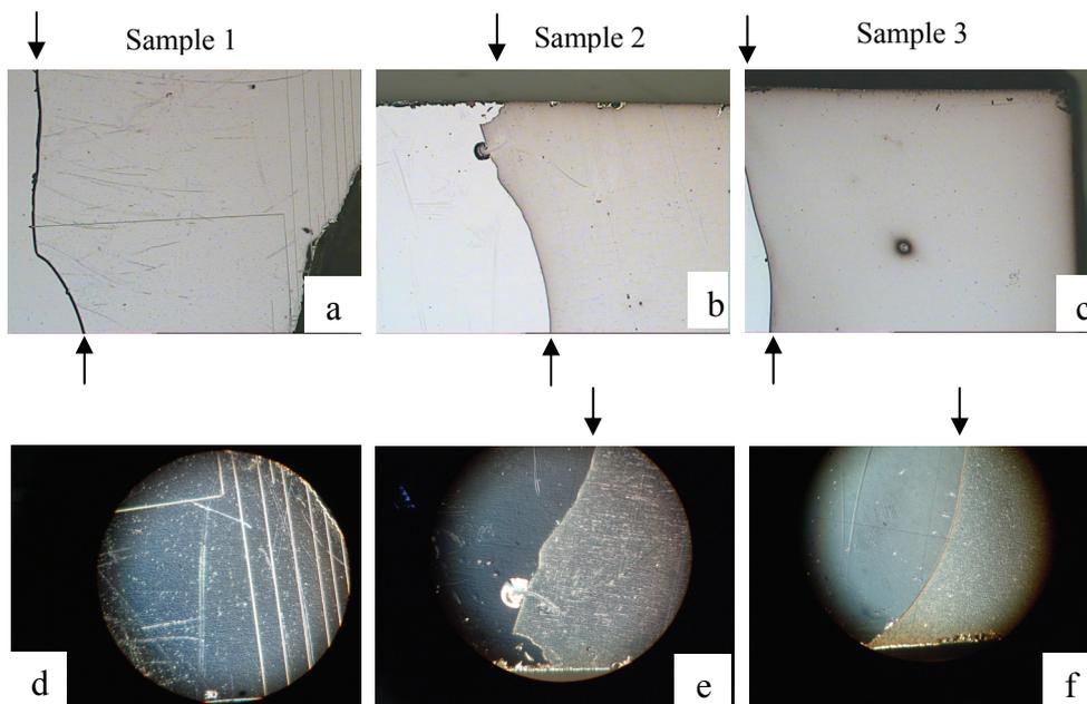
Fig. 1.16. Optical microscope images of  $\text{In}_x\text{Ga}_{1-x}\text{As}$  heterostructures ( $500 \mu\text{m} \times 380 \mu\text{m}$ ) in absence (a, b and c) and presence (d, e and f) of Nomarski contrast. Arrows show the borders of chemical etching.
