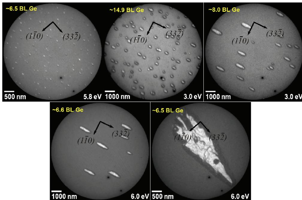
Fig. 1.14. The LEEM patterns of the Ge/Si(113) interface at different substrate temperatures (1 -  $380^\circ\text{C}$ ; 2 -  $440^\circ\text{C}$ ; 3 -  $490^\circ\text{C}$ ; 4 -  $540^\circ\text{C}$ ; 5 -  $590^\circ\text{C}$ ), thicknesses of Ge layers (1 - 6.5 bi-layer, 2 - 14.9 monolayer, 3 - 8 monolayer, 4 - 6.6 monolayer, 5 - 6.5 monolayer), electron energies (eV) 1 - 5.8; 2 and 3 - 3.0; 4 and 5 - 6.0, scanning areas of sample ( $\mu\text{m}^2$ ), 1 - 4 - 12.4; 5 - 6.2 [46].
