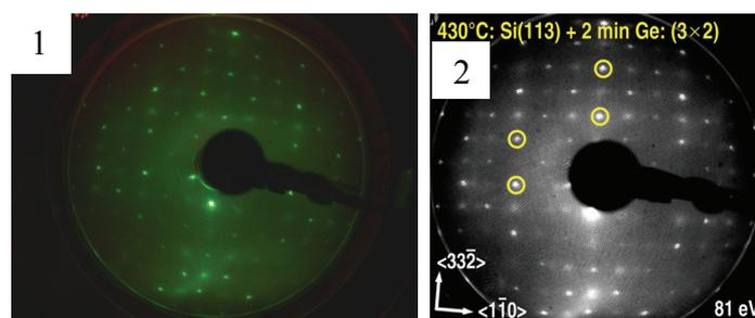
Fig. 1.6. The LEED patterns of Si(113)-3×2 reconstruction, after 2 minutes' Ge deposition at 430°C sample temperature. Electron energies are 53 eV (1), 81 eV (2).
