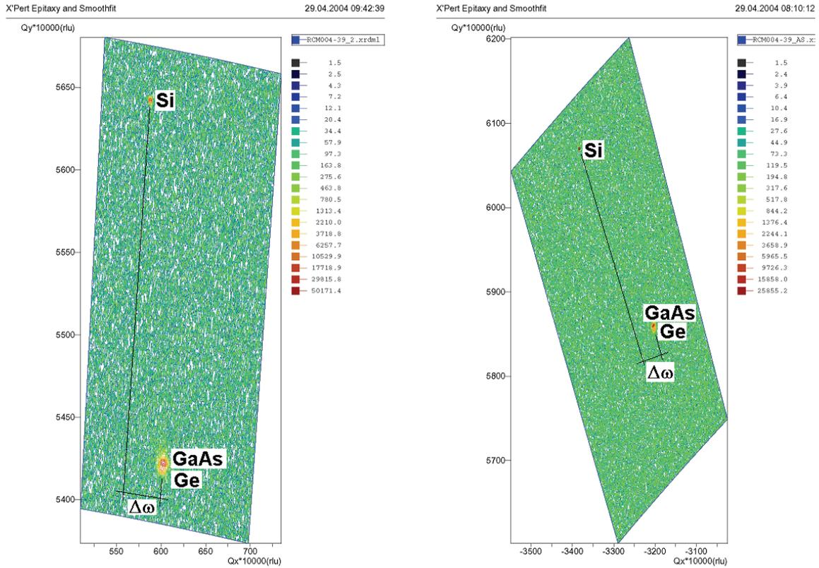
Fig. 1.18. The reciprocal space map of the heterostructure GaAs/  $\text{In}_x\text{Ga}_{1-x}\text{As}/\text{Ge}/\text{Si}(001)-6^\circ$  off towards  $[110]$  direction near 004 and 224 reflections.  $\Delta\omega$  is the tilt between crystal planes of the substrate and epilayers resulting from the miscut of the substrate
