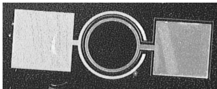
Fig. 1.21. Chemically etched structure of the monolithically integrated  $p^+$ -GaAs/n-GaAs/ $n^+$ -GaAs solar cell on silicon substrate with high crystallographic index, ohmic contacts of 1 - Ge and 2 - GaAs epilayers.
