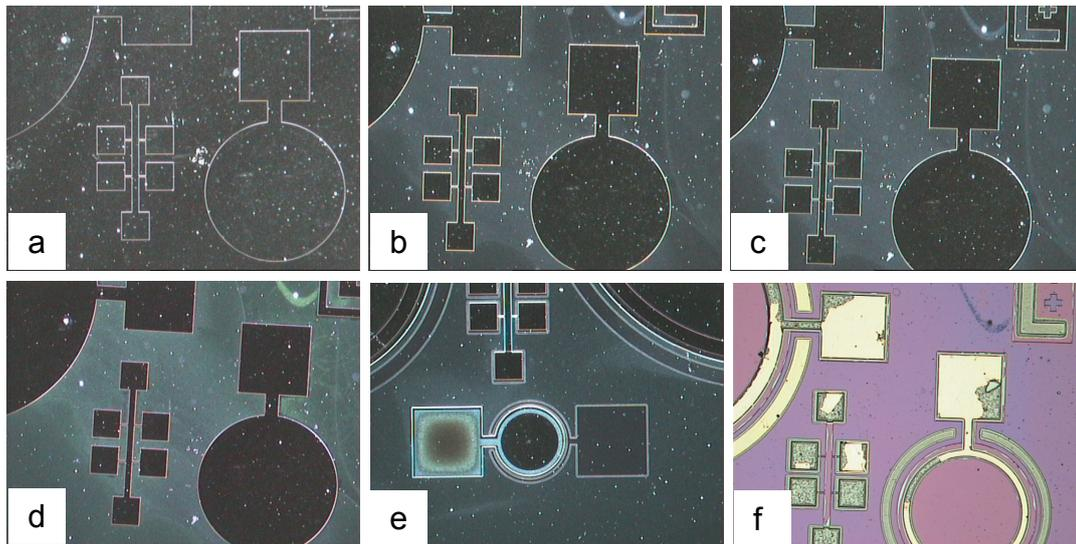
Fig. 1.20. Optical microscope images of photolithography steps of elaboration of the monolithically integrated  $p^+$ -GaAs/n-GaAs/ $n^+$ -GaAs solar cell on silicon substrate with high crystallographic index: a) photoresist deposition for mesa formation, b) development and removal of exposed photo-resist, c) mesa formation by etching, d) photoresist deposition for contact formation, e) development and removal of exposed photoresist, f) metal deposition.
