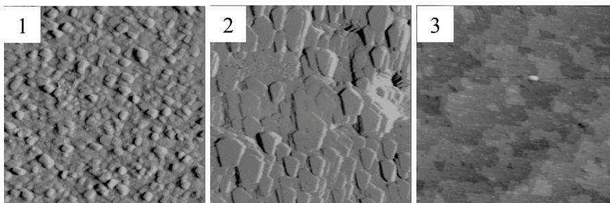
Fig. 1.12. The STM images of the Si(113)- $3\times 2$  (1 and 2) surface and the Si(113):Sb (3) interface with the Ge coverage at different temperatures and areas at voltage applied to the sample - 3 V, tunneling current - 0.5 nA, 1) 430°C ( $1000 \text{ nm}^2$ ), 2) 600°C ( $1000 \text{ nm}^2$ ), 3) 600°C ( $200 \text{ nm}^2$ )
