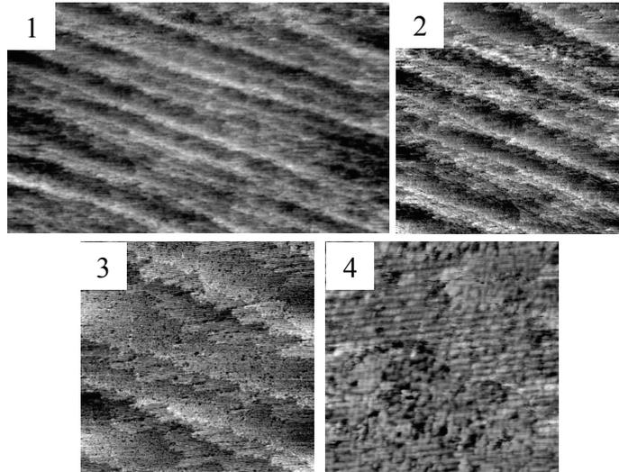
Fig. 1.10. The STM images of the Si(113)- $3\times 2$  surface with Ge coverage at different areas ( $\text{nm}^2$ ) at 430°C substrate temperature, deposition time of Ge - 30 min, voltage applied to the sample - 2 V, tunneling current - 0.3 nA, 1 -  $1000 \times 600$ , 2 -  $500 \times 500$ , 3 -  $200 \times 200$ , 4 -  $70 \times 70$
