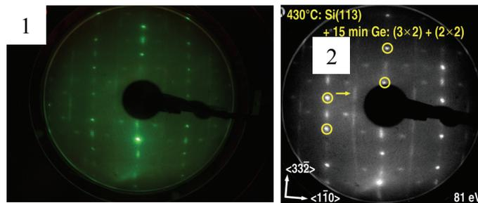
Fig. 1.8. The LEED patterns of Si(113)- $3 \times 2/3 \times 1$  reconstructions, after 15 minutes' Ge deposition at  $430^\circ\text{C}$  sample temperature. Electron energies are  $53 \text{ eV}$  (1),  $81 \text{ eV}$  (2).
