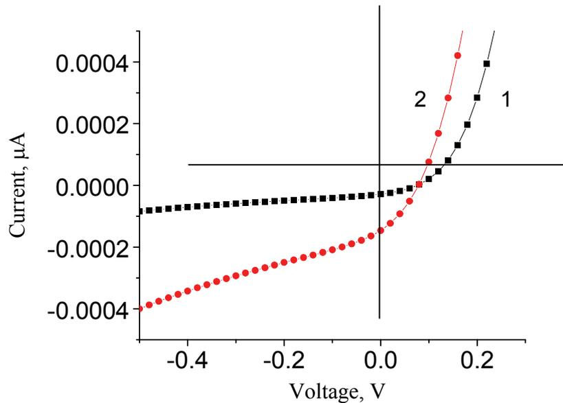
Fig. 1.23. I-V curves of two samples of the monolithically integrated  $p^+$ -GaAs/n-GaAs/ $n^+$ -GaAs solar cells on silicon substrate with high crystallographic index.
