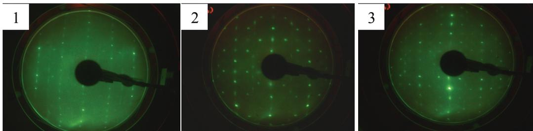
Fig. 1.11. The STM images of Si(113)- $3\times 2$  surface with Ge coverage at different electron energies and at 430°C substrate temperature after 30 minutes Ge deposition (eV), 1 - 53, 2 - 81, 2 - 130
