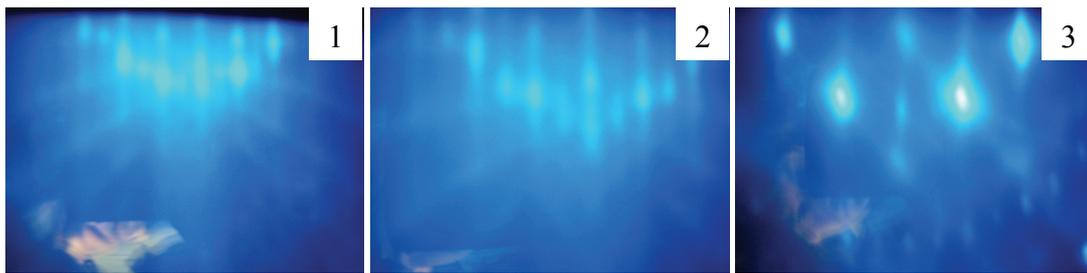
Fig. 1.13. The RHEED patterns of Ge/Si(113) interface at different crystallographic directions 1 - [110], 2 -  $[\bar{1}10]$ , 3 - [010]
