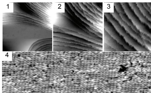
Fig. 1.1. The STM images of the clean surface of Si(113)-3×2 reconstruction. The scan areas are 1000 nm × 1000 nm (1), 500 nm × 500 nm (2), 250 nm × 250 nm (3), 56 nm × 13 nm (4) using sample voltage of -2 V and tunnelling current of 0.3 nA.
