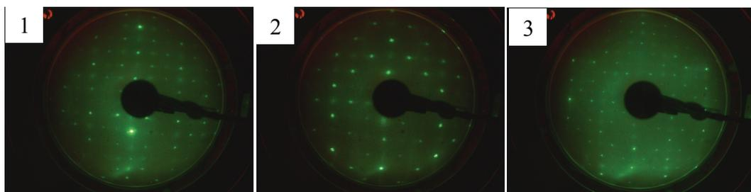
Fig. 1.4. The LEED patterns of Si(113) reconstructions, after 15 minutes' Ge deposition at 300°C sample temperature. Electron energies are 53 eV (1), 81 eV (2), 130 eV (3).
