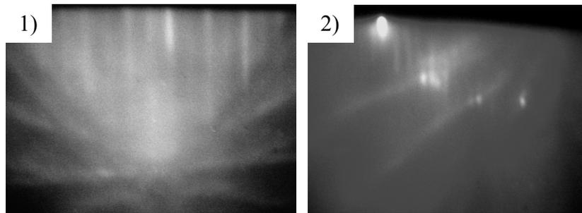
Fig. 1.19. The RHEED images of GaAs/ $\text{In}_x\text{Ga}_{1-x}\text{As}/\text{Ge}/\text{Si}$  heterostructure at different crystallographic directions; 1 -  $[110]$  and 2 -  $[-\bar{1}10]$
