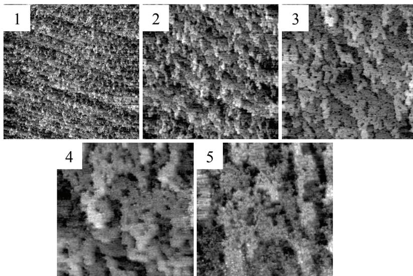
Fig. 1.3. The STM images of the Si(113) surface after 15 minutes' Ge deposition grown at 300°C, The scan areas are 1000 nm × 1000 nm (1), 500 nm × 500 nm (2), 150 nm × 150 nm (3), 100 nm × 100 nm (4), 75 nm × 75 nm (5) using sample voltage of - 2 V and tunneling current of 0.3 nA.
