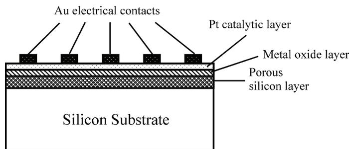
Fig. 1 Schematic diagram of gas sensor
