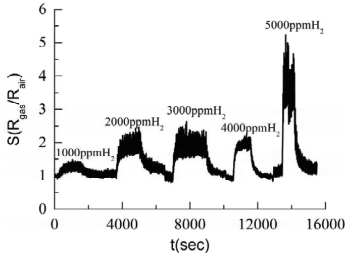
Fig. 4 Sensitivity of PS/TiO<sub>2-x</sub>/Pt structures to different concentration of hydrogen at 40°C
