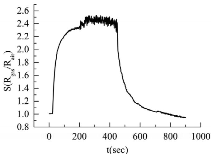
Fig. 3 Sensitivity of PS/TiO<sub>2-x</sub>/Pt structures at room temperature
