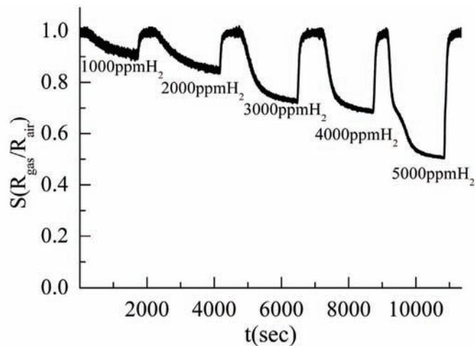
Fig. 5 Sensitivity of PS/ZnO<Al>/Pt structures to different concentration of hydrogen at 40°C
