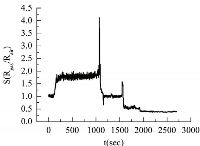
Fig. 2 Sensitivity of porous silicon structures to 5000 ppm hydrogen vs. time
