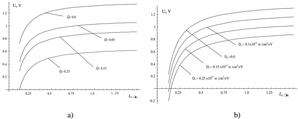
Fig.2. Threshold voltage versus channel length for different values of traps concentration (a) and surface states concentration (b).
