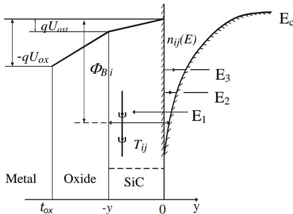
Fig. 1. Band diagram of the SiC- SiO2 system in the presence of a trap.
