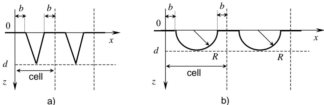
Fig. 1. Schematic illustrations of porous cells with conical (a) and spherical (b) configurations.
