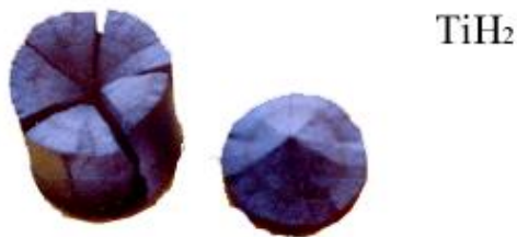
Fig. 3. Photo of non-crushed SHS-synthesized \text{TiH}_2 sample.
