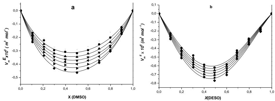
Fig. 1 Excess molar volumes,  $V_m^E \times 10^6 \left( m^3 mol^{-1} \right)$ , of binary solutions of AN at  $T=(298.15-323.15) K$ : (a) AN-DMSO; (b) AN-DESO, 298.15K (●); 303.15K (▲); 308.15K (▼); 313.15K (◀); 318.15K(►); 323.15K (◆).
