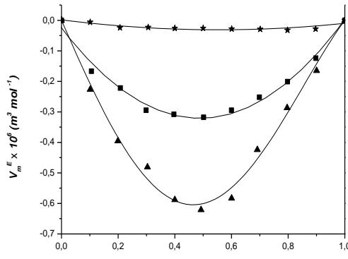
Fig. 2- Excess molar volumes,  $V_m^E \times 10^6 \left( m^3 mol^{-1} \right)$ , of binary solutions of AN at  $T=298.15K$ : (■) AN-DMSO; (▲) AN-DESO; (★) AN-ACN.
