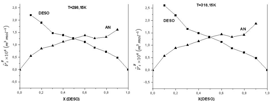
Fig. 4 Excess partial molar volumes,  $\bar{V}_i^E \times 10^6 (m^3 mol^{-1})$ , of components in binary solutions of AN at  $T = (298.15 \text{ and } 318.15) \text{ K}$ : (a) AN-DMSO; (b) AN-DESO.
