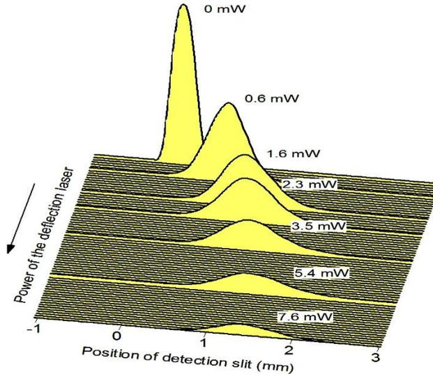
Fig 4 Transversal position  $\Delta x$  of atomic beam 89 cm downstream the interaction with deflection laser radiation depending on its power. The vertical scale shows the intensity of fluorescence excited by the detection laser.
