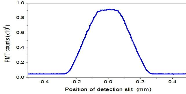
Fig 3 Typical downstream spatial profile of the atomic beam in the absence of the deflection laser. The full width at half-maximum is  $\approx 0.3$  mm.
